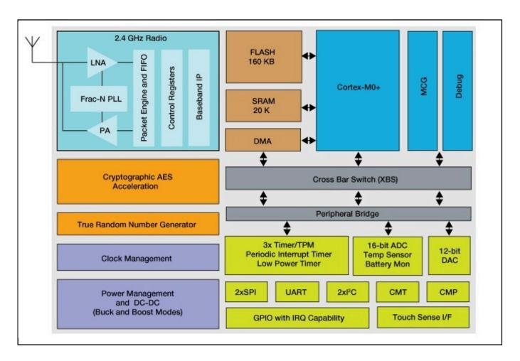
View additional information for Kinetis® KW40Z-2.4 GHz Dual Mode: Bluetooth Low Energy and 802.15.4 Wireless Radio Microcontroller (MCU) based on Arm® Cortex®-M0+ Core.
