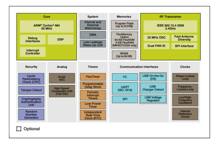
View additional information for Kinetis® KW2xD-2.4 GHz 802.15.4 Wireless Radio Microcontroller (MCU) based on Arm® Cortex®-M4 Core.
