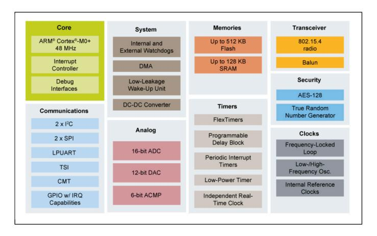
View additional information for Kinetis® KW21Z-2.4 GHz 802.15.4 Wireless Radio Microcontroller (MCU) based on Arm® Cortex®-M0+ Core.
