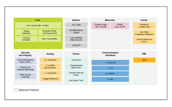
View additional information for Kinetis® KV1x-75 MHz, Entry-Level 3ph FOC / Sensorless Motor Control MCUs based on Arm® Cortex®-M0+.
