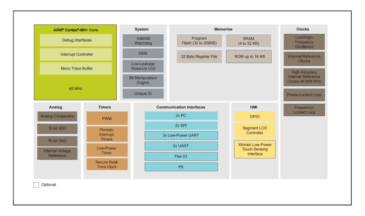
View additional information for Kinetis® KL3x-48 MHz, Segment LCD Ultra-Low-Power Microcontrollers (MCUs) based on Arm® Cortex®-M0+ Core.
