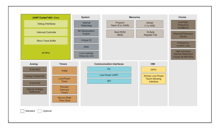
View additional information for Kinetis® KL0x-48 MHz, Entry-Level Ultra-Low Power Microcontrollers (MCUs) based on Arm® Cortex®-M0+ Core.
