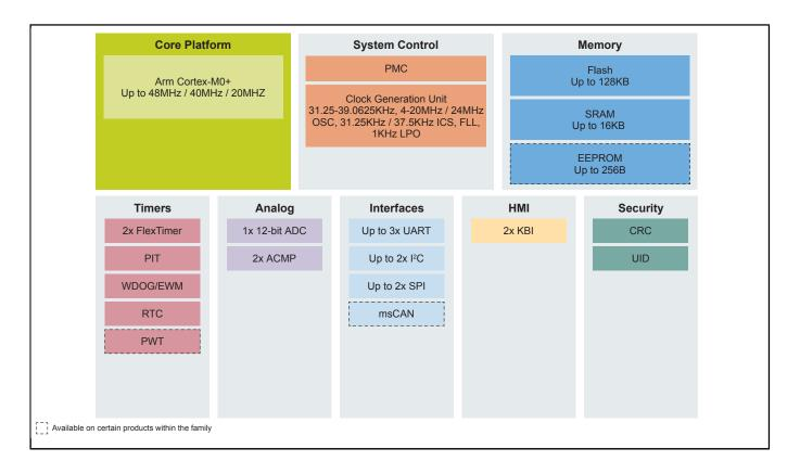
View additional information for Kinetis® KE06-48 MHz, Mainstream with CAN Microcontrollers (MCUs) based on Arm® Cortex®-M0+ Core.
