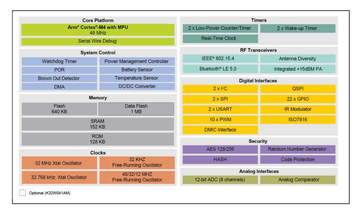
View additional information for K32W041AM/A: High Performance, Secure and Low-Power MCU for Zigbee®, Thread<sup>™</sup> and Bluetooth® LE 5.0 with High Tx Power Option.
