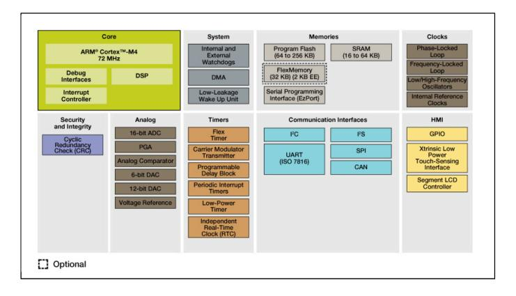
View additional information for Kinetis K30-72 MHz, Mixed-Signal Integration Microcontrollers (MCUs) based on Arm® Cortex®-M4 Core.
