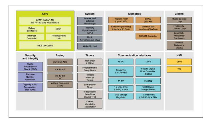
View additional information for Kinetis® K26-180 MHz, Dual High-Speed and Full-Speed USBs, 2MB Flash Microcontrollers (MCUs) based on Arm® Cortex®-M4 Core.
