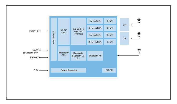
View additional information for 2.4/5 GHz Dual-Band 2x2 Wi-Fi® 6 (802.11ax) + Bluetooth® 5.1 Solution.
