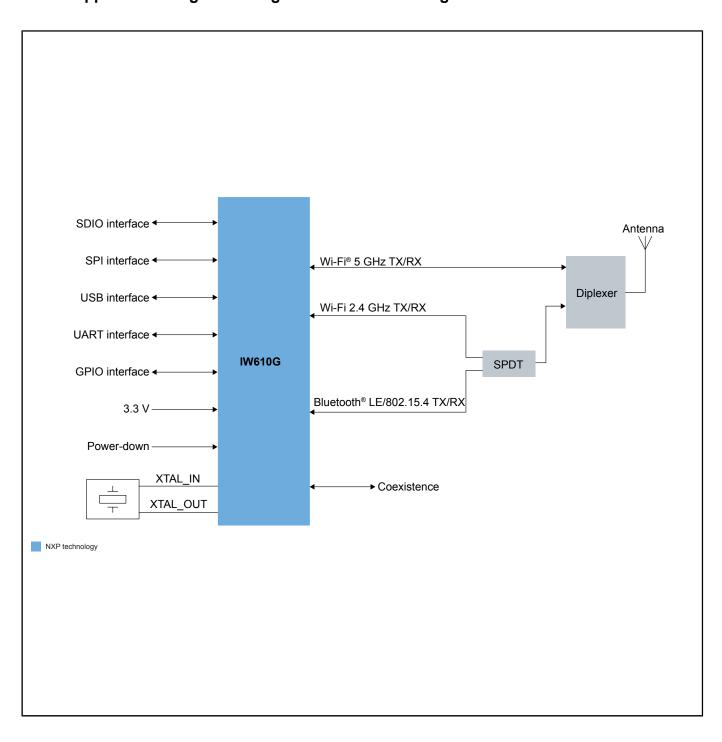
IW610 Application Diagram - Dual Antenna Block Diagram
