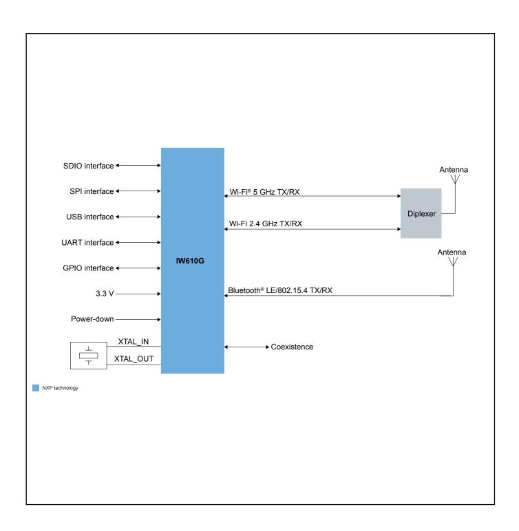
IW610 Internal Block Diagram Block Diagram
