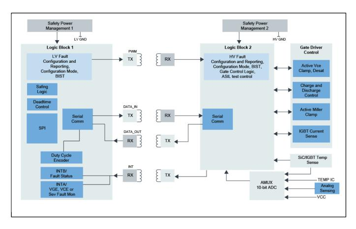
View additional information for Advanced High Voltage Isolated Gate Driver with Segmented Drive for SiC MOSFETs.
