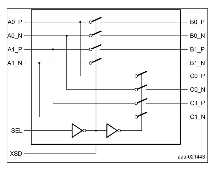
View additional information for High-Speed Differential 1-to-2 Switch Chip.
