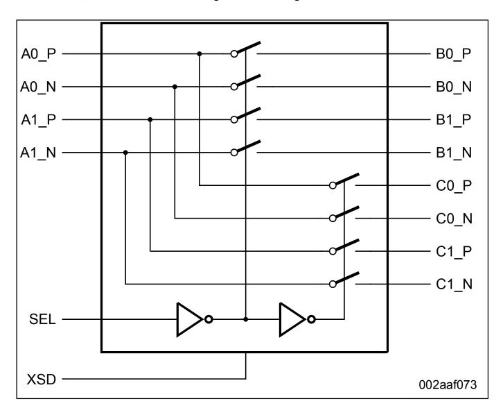
View additional information for 3.3 V, Two Differential Channel, 2-1 Multiplexer/Demultiplexer Switch for PCI Express® Gen2.
