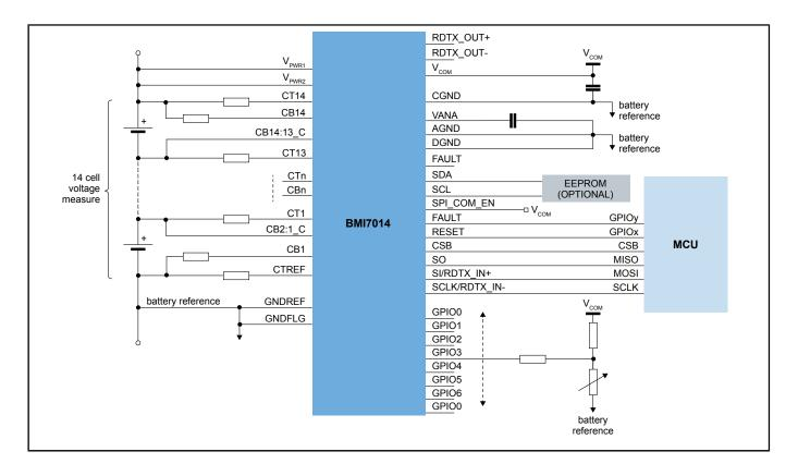
View additional information for 14-Channel Li-Ion Battery Cell Controller IC.
