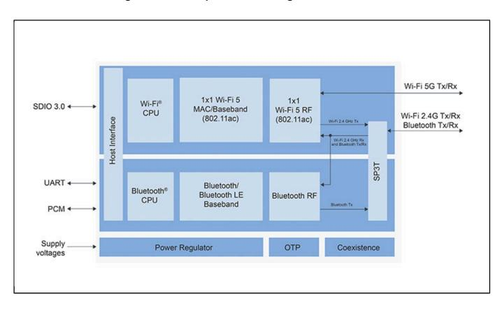
View additional information for 2.4/5 GHz Dual-Band 1x1 Wi-Fi® 5 (802.11ac) + Bluetooth® 5.2 Solution.
