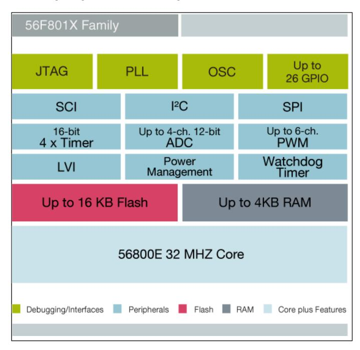
View additional information for Digital Signal Controller for Motor Control Applications.
