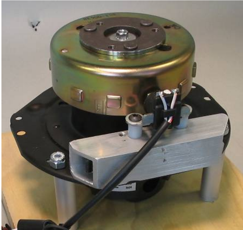
Figure 8. Spin Bench Example for Creating a Physical Simulated Engine Position Signal
