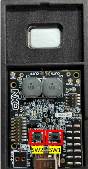
Figure 11. SW1 and SW2 on the SLN-LOCAL-IOT Kit.
