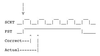
The correct time to latch the FST is on the falling edge when the clock polarity bit is clear. However, when SCKT trails FST it is actually being latched on the following rising edge as shown.
