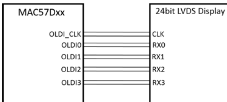
Figure 25. LVDS Connection with 24bit color display
