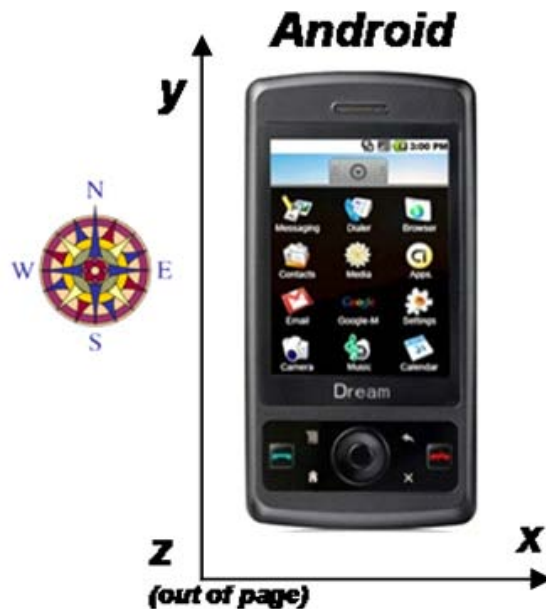
Figure 1. Android Coordinate System for 3-axis Accelerometer
