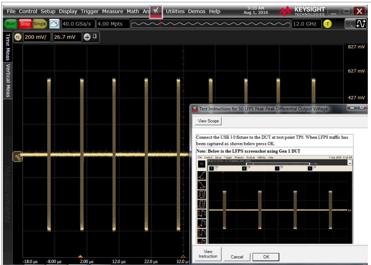
Figure 111. LFPS Signal in Test
