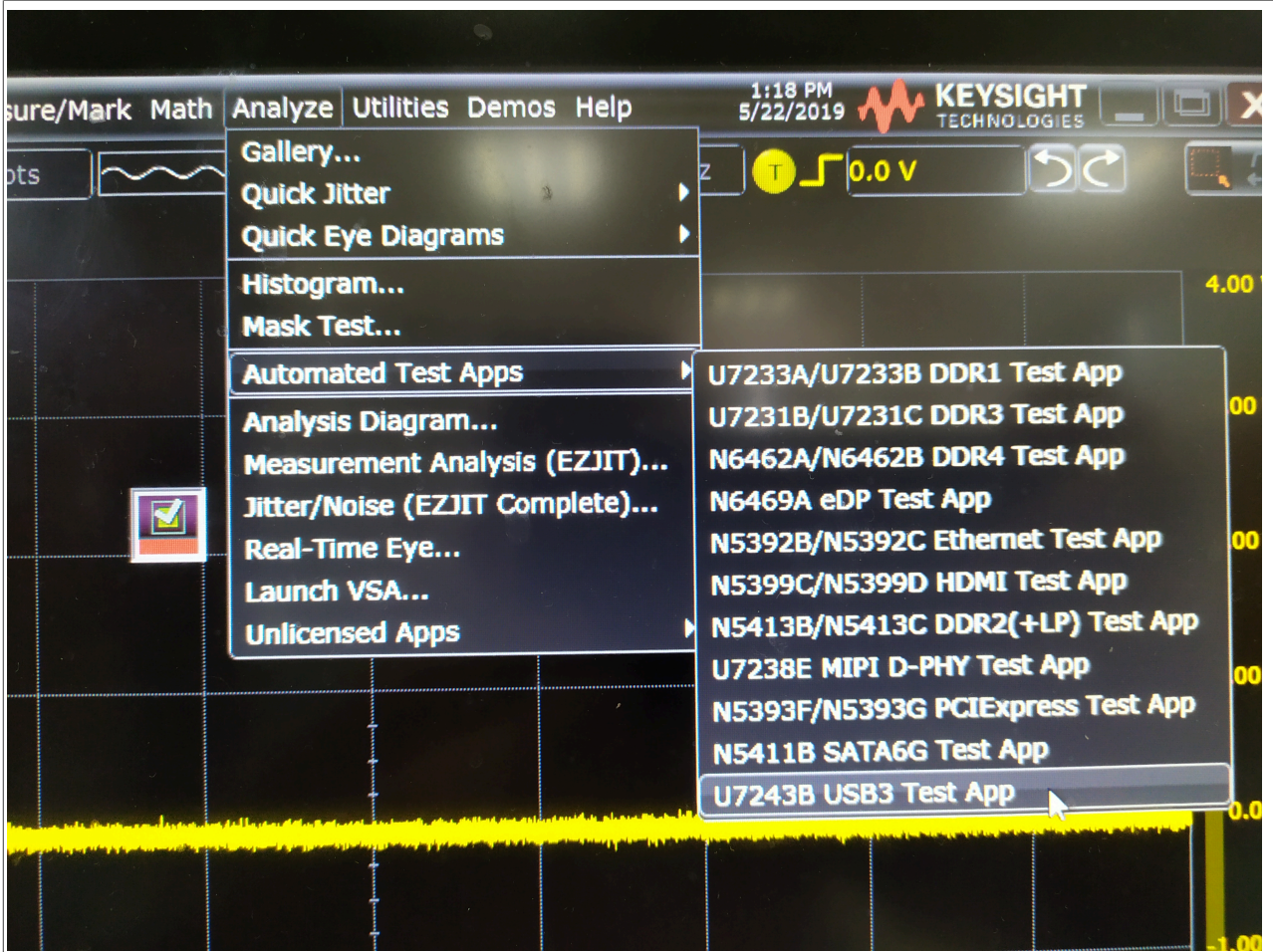
Figure 82. Automated Test Software for USB 3.0
