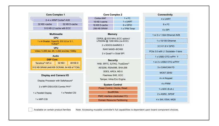
View additional information for i.MX 8X Family – Arm® Cortex®-A35, 3D Graphics, 4K Video, DSP, Error Correcting Code on DDR.
