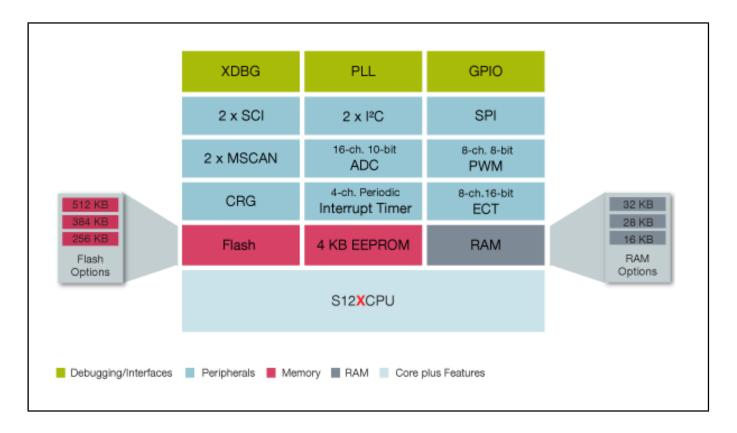
View additional information for S12XHZ Scalable Instrument Clusters Microcontrollers (MCUs) with CAN.
