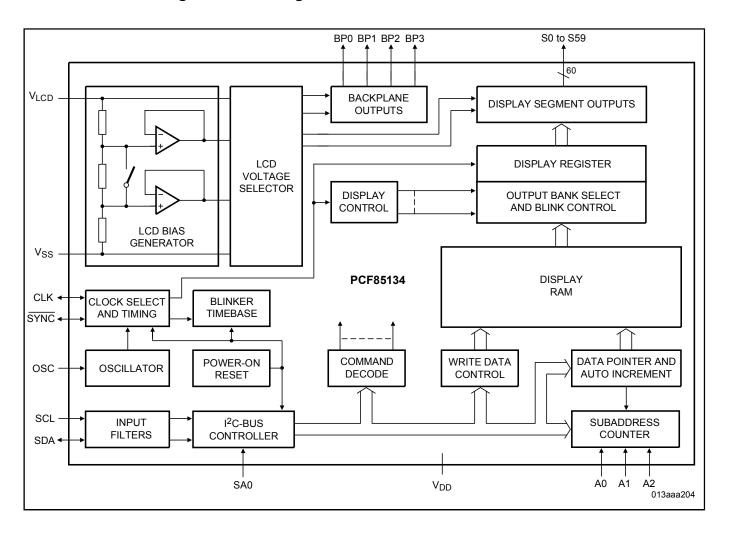
View additional information for Universal 60 X 4 LCD Segment Driver for Multiplex Rates Up to 1-4.
