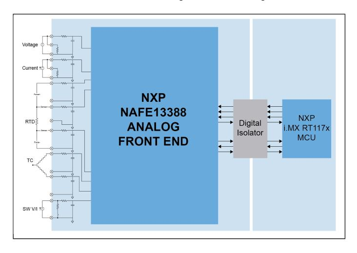
View additional information for Highly Configurable 8 Channel ±25 V Universal Input Analog Front-End with Excitation Sources.
