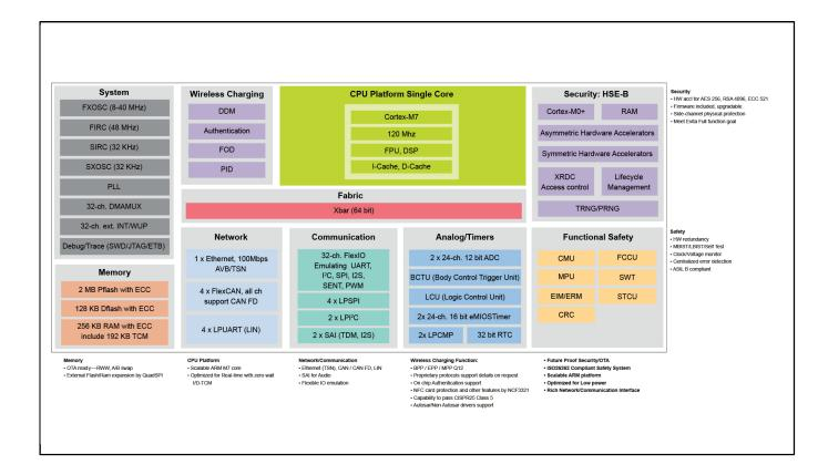
View additional information for MWCT2xxxS Microcontroller for Wireless charging Transmitter ICs.
