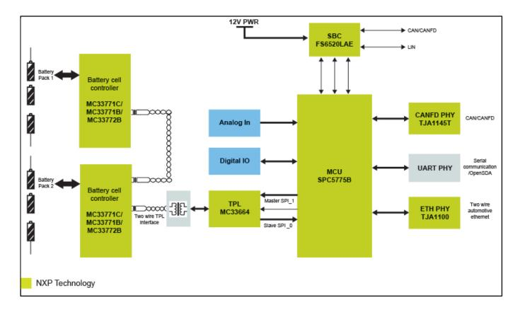
View additional information for MPC5775B and MC33771 high-voltage BMS Evaluation System.
