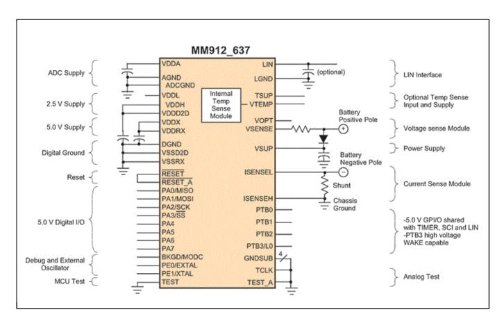
View additional information for Battery Sensor with LIN for 12 V Lead-Acid Batteries.
