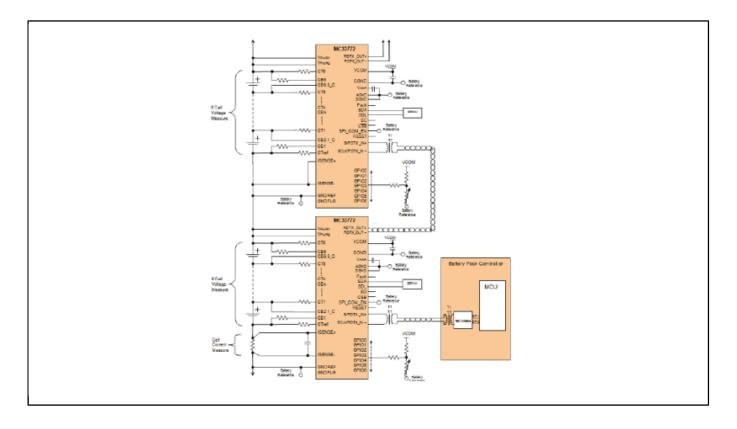
View additional information for 6-Channel Li-lon Battery Cell Controller IC.
