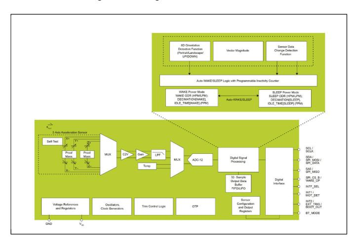
View additional information for ±2g/±4g/±8g/±16g, Low Power 12-bit Digital Accelerometer.
